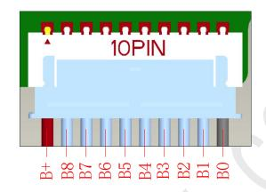
相关说明: 采样排线的走线排布不要扯太紧,以免使用过程中拉扯松脱; 主板插座和排线结合处要打胶固定。 Instructions: The routing of the sampling wiring harness should not be too tight to avoid being pulled loose during use; the junction between the motherboard socket and the wiring harness should be secured with adhesive.
