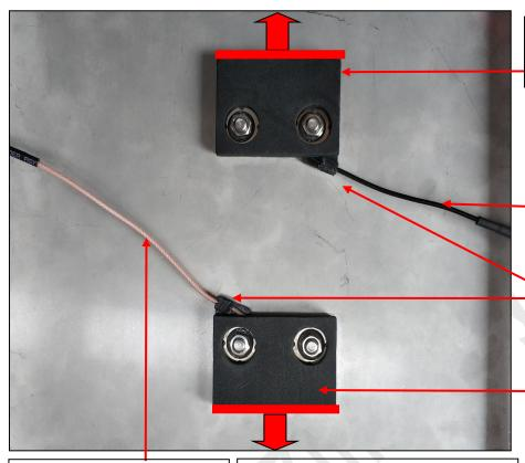
棕线为GSM天线 The brown one is a GSM antenna. 注意: GSM天线与把手的 "M" 对应 Note: The GSM antenna corresponds to the "M" of the handle.
