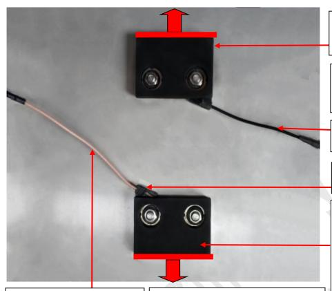
棕线为GSM天线 The brown one is a GSM antenna 注意: GSM天线与把手的"M"对应 Note: The GSM antenna corresponds to the "M" of the handle 注意:钢片天线的横梁朝外安装
