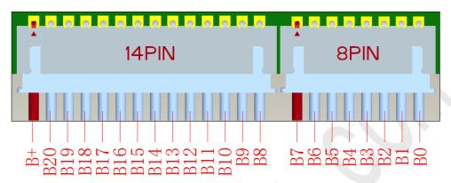
相关说明:采样排线的走线排布不要扯太紧,以免使用过程中拉扯松脱;主板插座和排线结合处要打胶固定。 Instructions: The routing of the sampling wiring harness should not be too tight to avoid being pulled loose during use; the junction between the motherboard socket and the wiring harness should be secured with adhesive.
