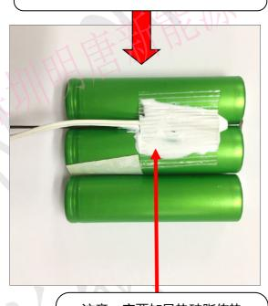
注意一定要加导热硅脂传热 Be sure to add thermal grease to heat transfer
