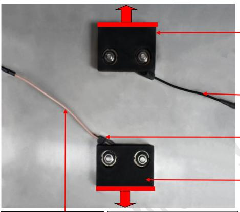
棕线为GSM天线 The brown one is a GSM antenna 注意: GSM天线与把手的"M"对应 Note: The GSM antenna corresponds to the "M" of the handle to the "S" on the handle
